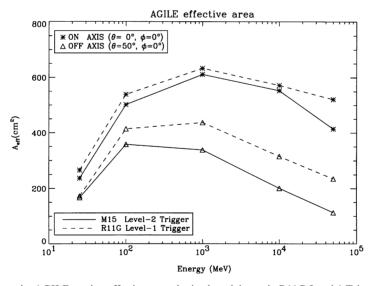
Fig. 9. Comparison between the AGILE-tracker effective area obtained applying only R11G Level-1 Trigger and the AGILE-tracker effective area obtained applying M15 Level-2 Trigger (after R11G+DIS).
