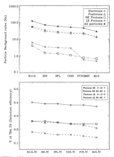
Fig. 1. Efficiency of the GRID Level-2/Step-1 data processing in rejecting particle background events (upper panel) and in detecting photons (lower panel). The suffix "TC" means "Tracker converted" (only photons converted in the tracker volume have been considered) and "FCN\_TC" means "FCN3MIP\_TC" (see text).
