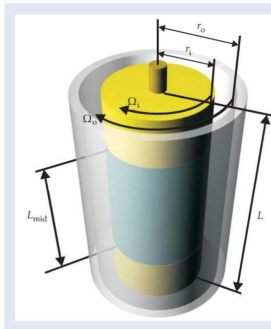
**Figure 1. A Taylor–Couette cell.** Water fills the gap between concentric cylinders, which are rotated with angular velocities  $\Omega_i$  and  $\Omega_o$ . To minimize the role of end effects, the new experiments measured only the torque on the middle length of the inner cylinder,  $L_{mid}$ . (Adapted from D. P. M. van Gils et al., <http://arxiv.org/abs/1011.1572>.)
