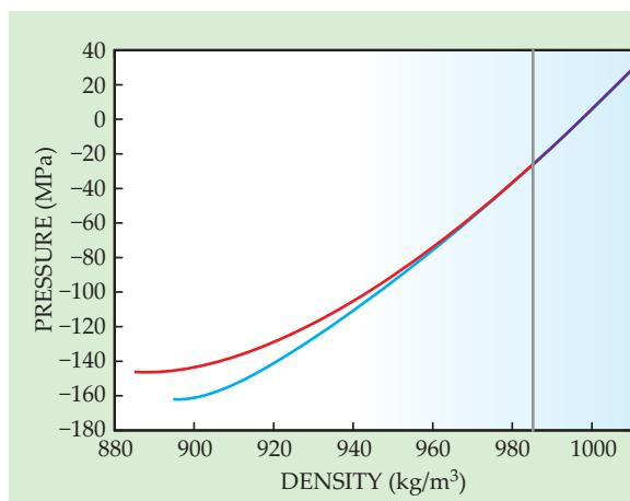
**Figure 3.** Water's equation of state as measured experimentally (purple) and extrapolated theoretically (red and blue). Although the ultrasound method can't generate tensions beyond  $-30$  MPa before vapor bubbles form, the measured equation of state agrees with models predicting that much greater tensions should be possible. (Adapted from ref. 1.)
